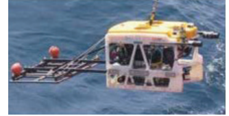
Survey skid with TSS pipe tracker
