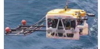
Survey skid with TSS pipe tracker
